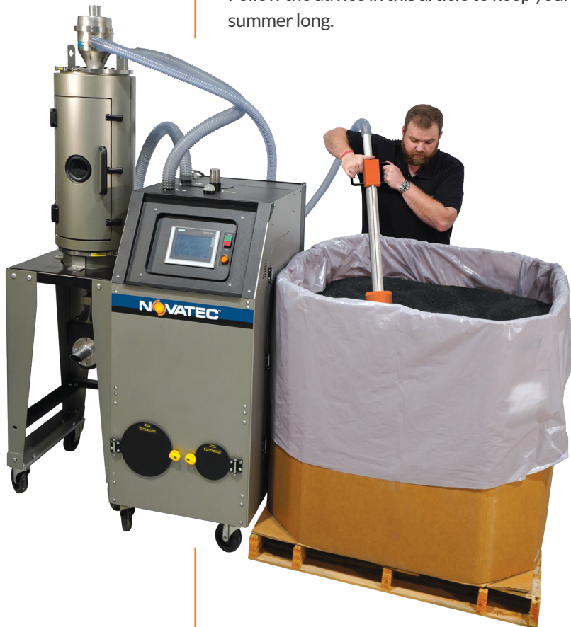
The DryerGenie by Novatec is a new offering in plastic moisture analyzing products and for the first time ever the dryer will know the exact moisture of the pellets prior to drying. Then, the program within the dryer control will automatically adjust the drying parameters so the plastic resin is dried to the prescribed moisture level in the shortest possible time with no operator intervention needed.
