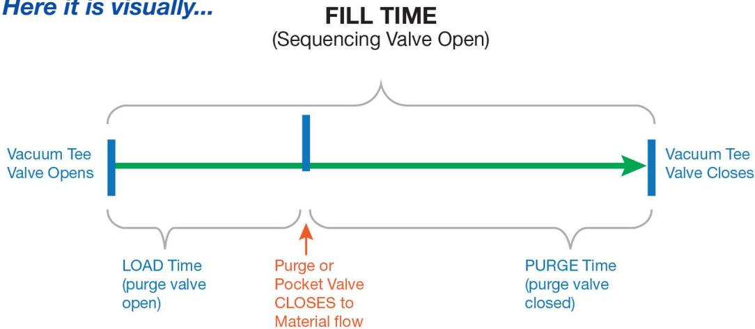
Note that it is common to set more PURGE time than LOAD time on the conveying control, to allow the entire conveying line to be cleaned of all pellets and even dust from the conveyed material.
